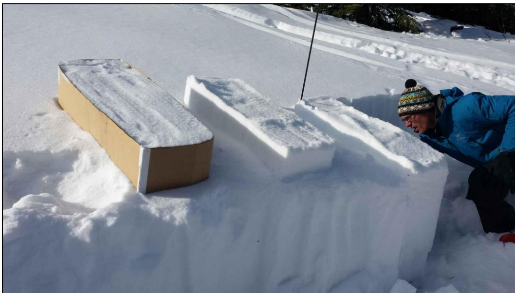
Figure 1: Here we've added slabs of 10, 15, and 20 cm to the snowpack (from right-to-left) and we are preparing the 10 cm slab for a PST. We allowed added snow to sinter for a minimum of 30 minutes.
