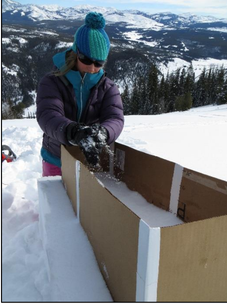
Figure 2: The most efficient technique for adding load to the snowpack proved to be adding disaggregated grains by hand to a cardboard frame, and then allowing those grains to sinter prior to testing.
