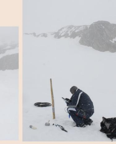
Each tag, after installation, has been interrogated and verified through the wireless communication using the MALATRA console.
