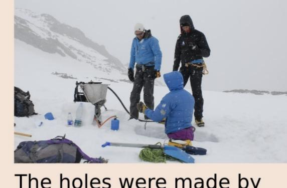
The holes were made by means of a steam driven ice drill
