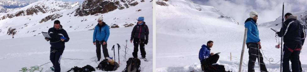
communication using a Yagi antenna: the maintenance of the RFID communication has been successfully checked up to a distance of approximately 100m.
